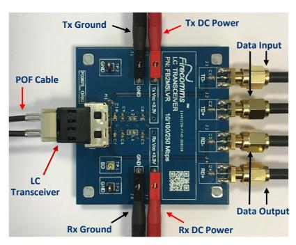
FIGURE 2 Setup of the FB2M5LVR Evaluation PCB
