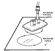
Place the 600 grit abrasive paper on a flat smooth surface, pressing down on the connector; polish the fiber and the connector using a figure eight pattern of strokes until the connector is flush with the bottom of the polishing fixture. Wipe the connector and fixture with a clean cloth or tissue.
