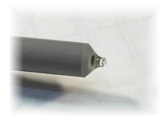
Insert the connector fully into the polishing fixture with the trimmed fiber protruding from the bottom of the fixture. This plastic polishing fixture can be used to polish two simplex connectors or simplex latching connectors simultaneously, or one duplex connector.
