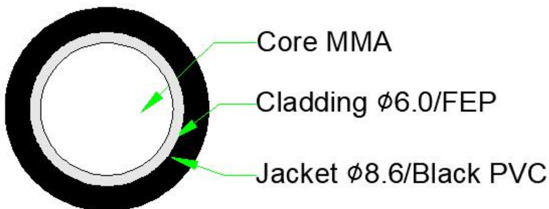
TX-SCC6000-1/8.6 Structure diagram
