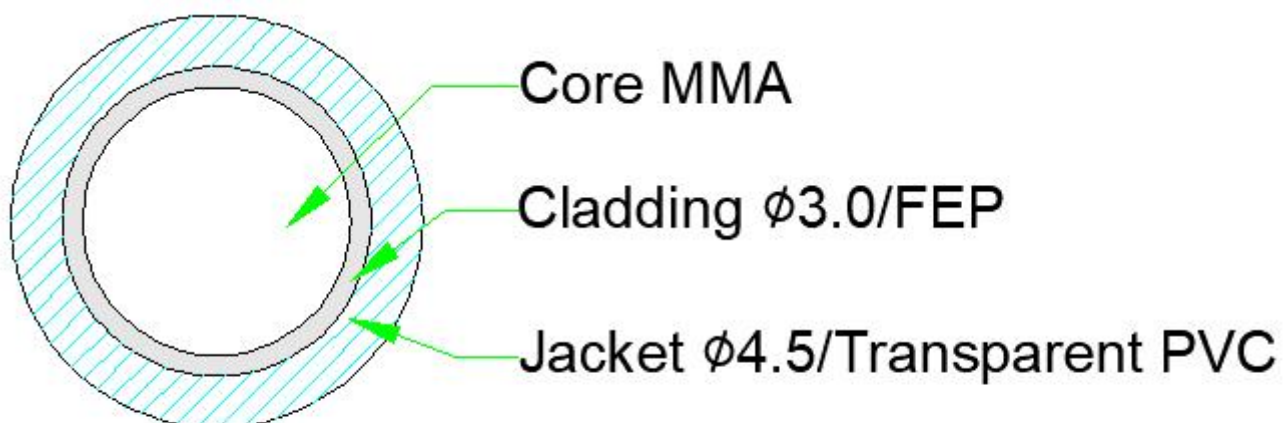
TX-SCC3000-1/4.5T Structure diagram
