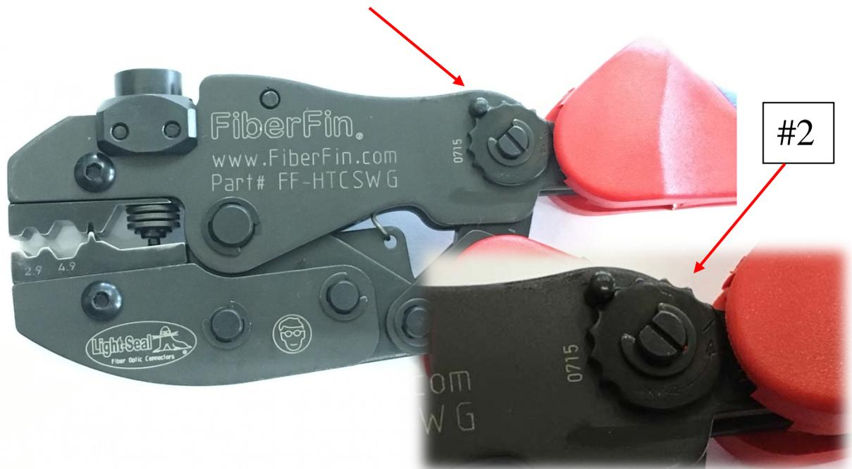
3. If the setting dial #2 is rotated clockwise + this configures a stronger crimp force and a smaller crimp height, (the smallest possible would be the hex size) regulation of the crimping force should not exceed 180 N
