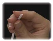
**Note:** The eye safe visible red light at the end of the fibre indicates the link is good. It can also be used to guides correct orientation when inserting the fibre into the connector.
