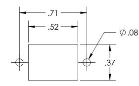
RECOMMENDED MOUNTING HOLE (SC SIDE) MAX THICKNESS: 0.067
