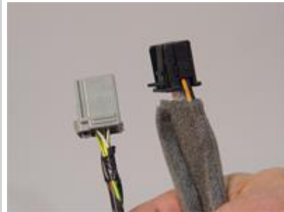
Figure 2 - From the side view these plugs look nearly alike.
