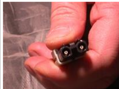
Figure 3 - When looking into the plug end, fiber-optics do not use common electrical terminal connectors.
