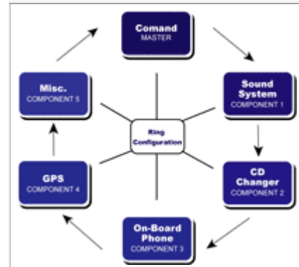
Figure 1 - A fiber-optic circuit must be connected in a loop to operate.
