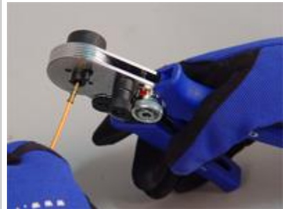
Figure 6 - Ferrules are installed with a special tool.
