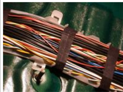
Figure 4 - Fiber-optic cables are not easily identifiable from copper wires.
