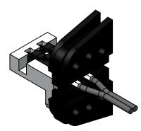
STEP 6: RELEASE THE CRIMPING TOOL AND THE FIBER REMAINS SECURE IN PLACE
