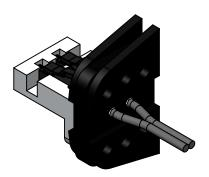
STEP 5: WHILE HOLDING THE FIBER IN PLACE, CRIMP THE END OF THE CONNECTOR
