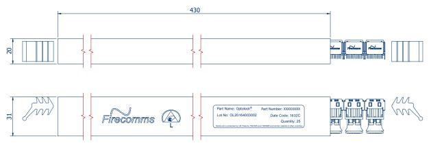
FIGURE 10 Packing tube for Firecomms OptoLock® Transceivers.
