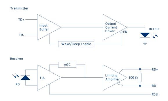
FIGURE 3 Electronic block diagrams of the Transmitter and Receiver fibre optic transceivers.
