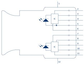
FIGURE 1 Transceiver pin-out numbering scheme, top view shown.
